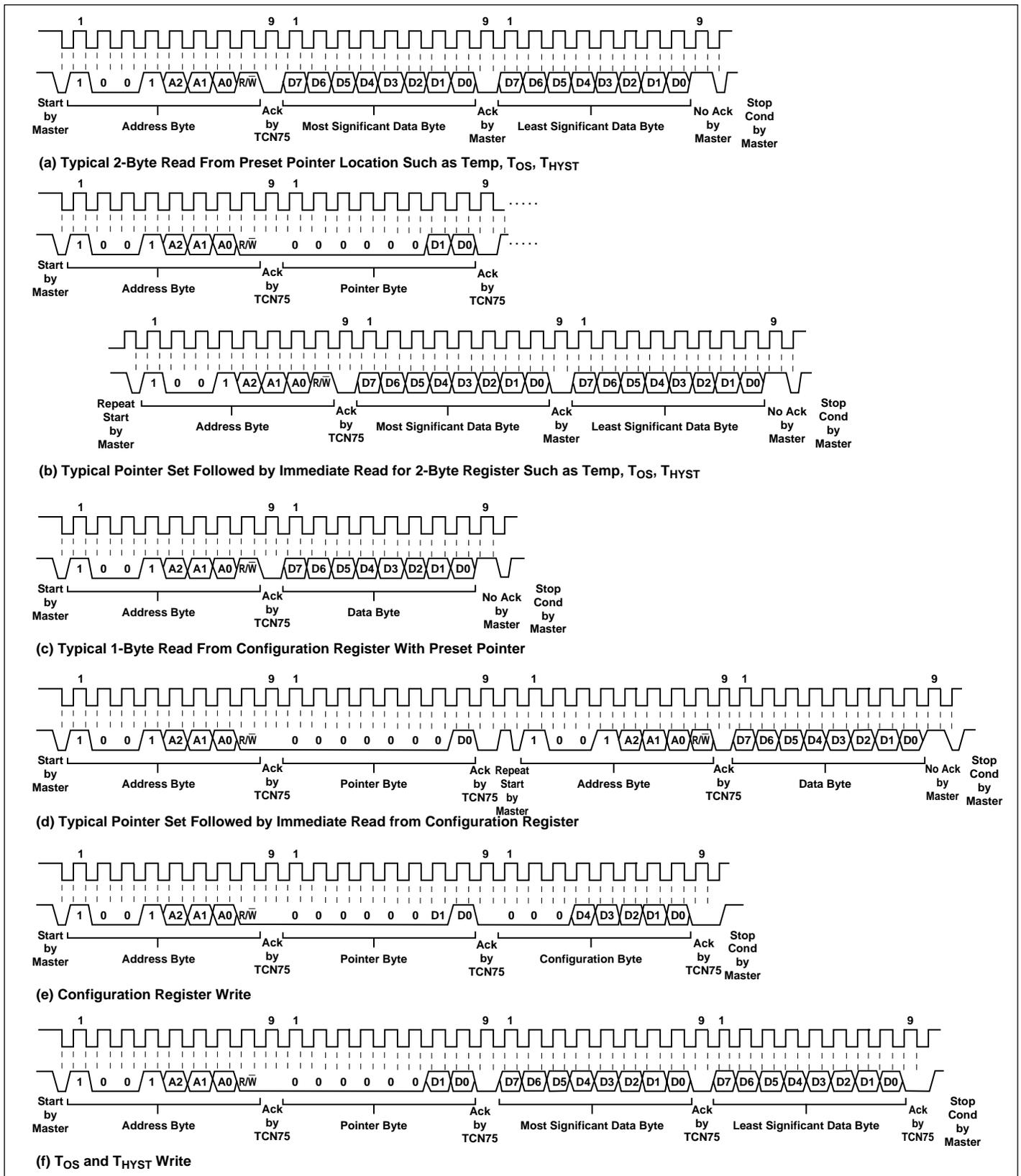
Figure 2. Timing Diagrams
